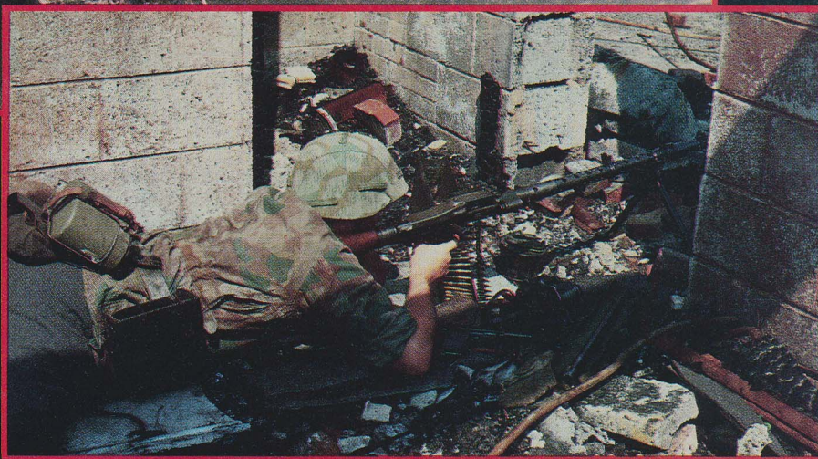
The MG34, which traced its beginning to Solothurn of Sweden, could be fed either by a belt or self-contained 75-round drum magazine. In many instances the MG34 was used as a squad light machine gun.
