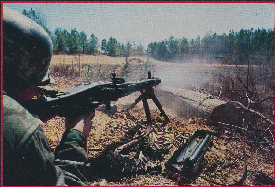
The MG42 used a roller locking bolt not unlike the Heckler and Koch assault rifles of today.
