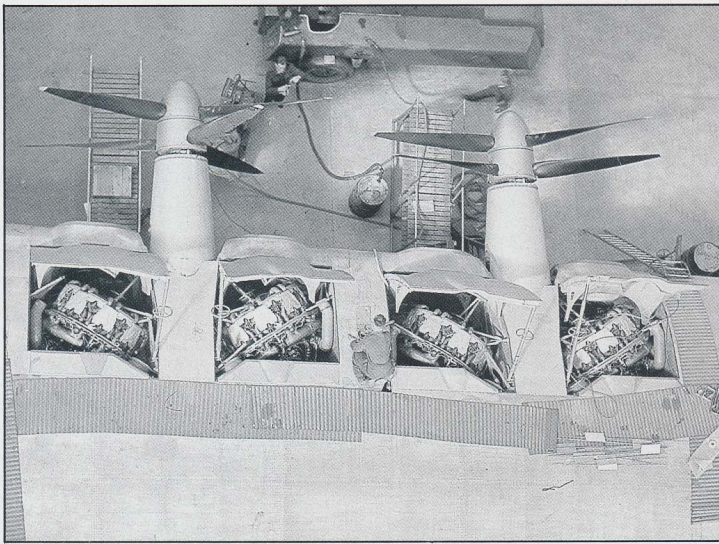
The Brabazon was powered by eight Bristol Centaurus 2650 hp engines coupled in pairs to drive contra rotating Rotol airscrews.
