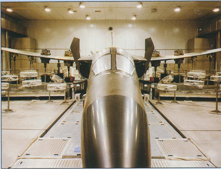
F-111 undergoing structural testing in the Cold Proof Test Chamber.
