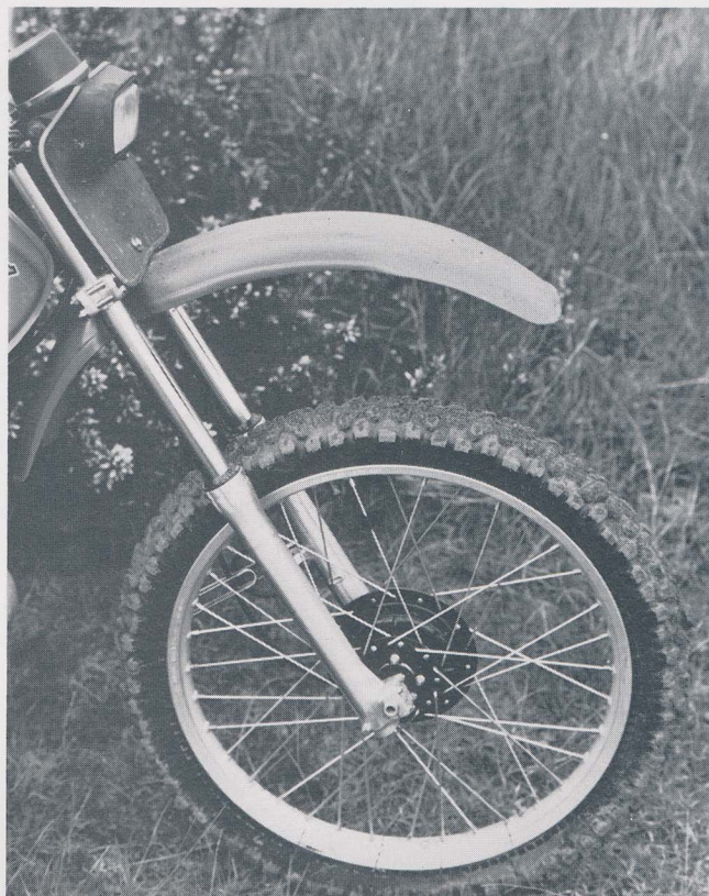
The dreaded 23in front wheel. One of the all-time great mistakes in Honda's design and marketing policies. The forks weren't too good either.
