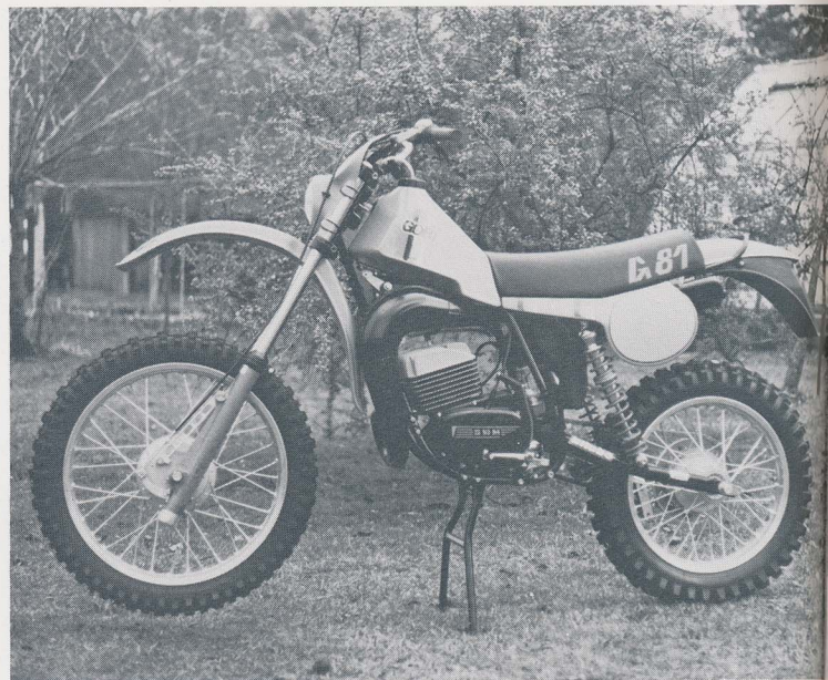
Not a surrogate SWM by any means – the Gori had its own very special characteristics. Humped tank and Samfis forks made the Gori unmistakable.
