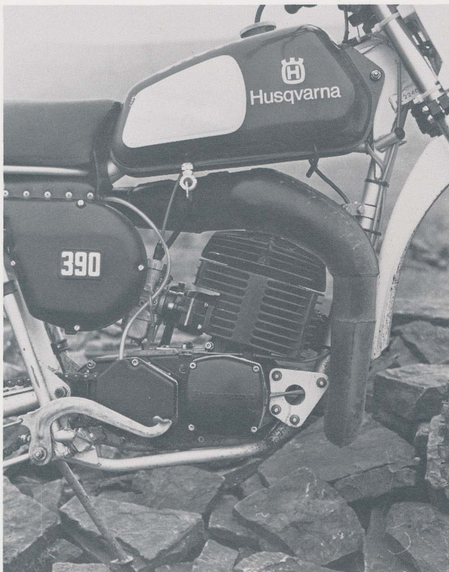
The Auto motor consists of a 390 motocross barrel and bottom half with the Husqvarna automatic gearbox housed in place of the conventional gearbox. By far the neatest arrangement of any automatic.
