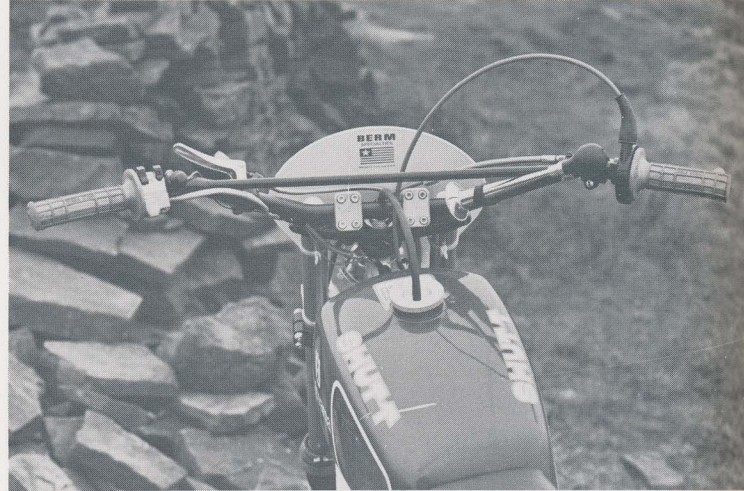
A sight familiar to all Husky Auto riders. The small lever on the left releases the drive and gets the bike in action.
