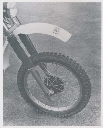
The once all British CCM had begun to buckle under the pressure to use foreign propietary parts of high quality and low cost. The front fork is the magnesium-slidered Marzocchi, whilst the front hub is by Grimeca — both equal to, or superior to, the earlier British made parts.
