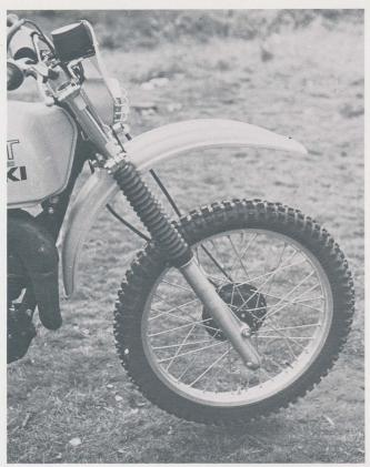
Although appearing to be more sophisticated, the 175 forks were, in practice, inferior to the 'old' 250 pattern which they superseded. Front brake was typical Suzuki – superb.
