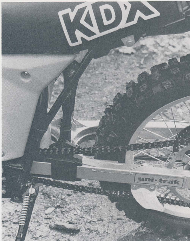
Unique Uni-Track rear end. The 175 enduro was the most successful application of this design in any of the Kawasaki off-road range.
