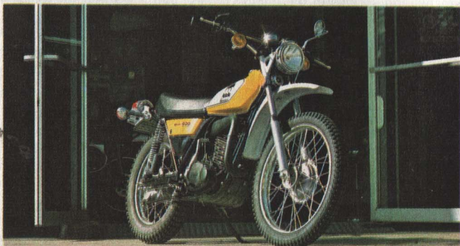
Enduro bikes, like the DT-400B, have great ground clearance; a strong bashplate protects the engine.
