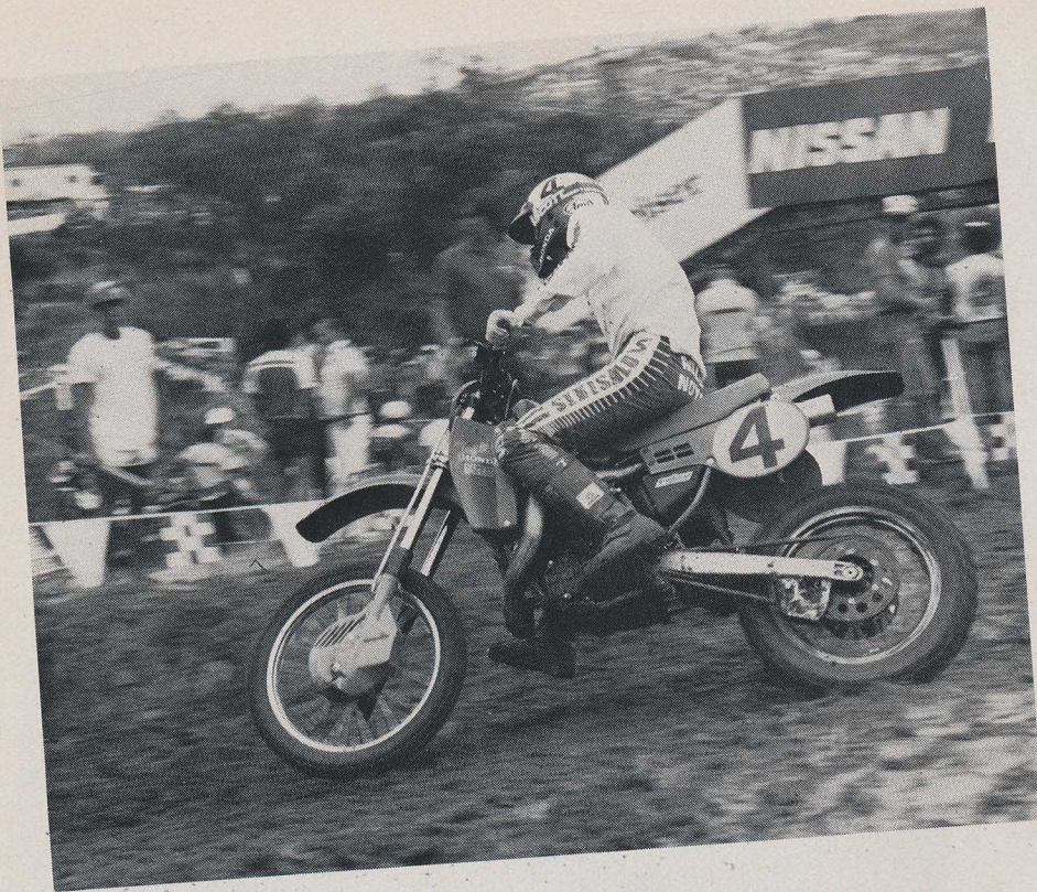
Graham pilots a liquid-cooled, disc-braked, ATAC-equipped RC500 works Honda at the GPs.
