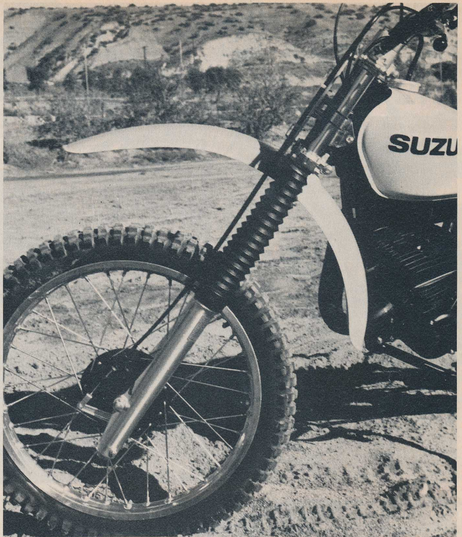
Leading axle forks are up to 9.1" of travel.
