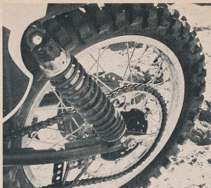
Kayaba gas shocks are undersprung and underdamped, but the pipe isn't too bad.
