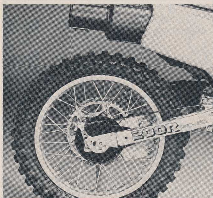
The rear suspension was too soft for our overweight testers. Extra preload helps.
