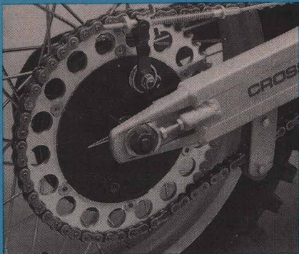
Non-floating, quick-change rear brake was trouble-free.
