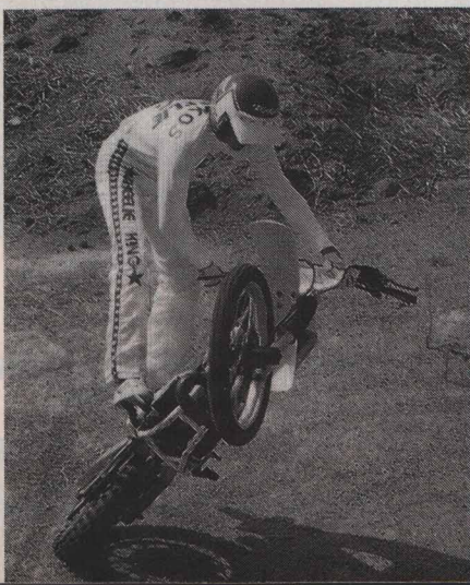
Doug leans his bike into the turn while remaining centered over his line. Steering inside makes the bike fall into the turn. Bike lean is then controlled by steering away from the turn.
