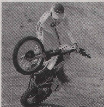
Increasing speed allows more bike lean, especially with a motor-driven front wheel. Note how Doug weights to the outside of the turn and countersteers to create an up-force against bike lean.
