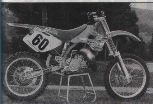
Noleen claims that the short silencer is responsible for some of the crisp low-rpm response, but it is definitely a little on the raspy side.
