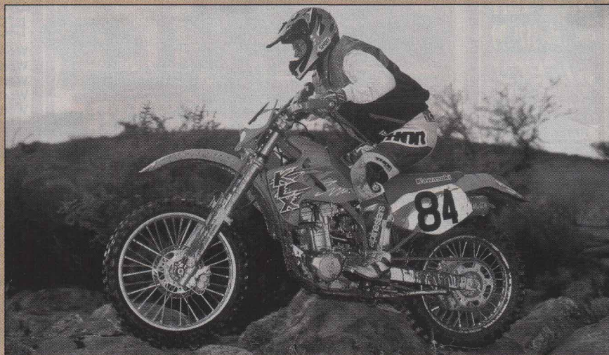
After switching to stiffer 0.42 kg/mm fork springs, we neglected to soften compression damping, and the front rode too high and stiff in the rocks.
