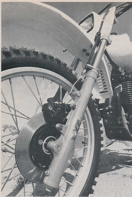
Brembo hydraulic disc provides smooth progressive action. Forks have 10.8 in. travel.
