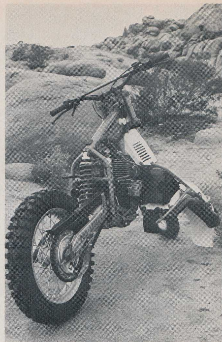
You can unbolt the rear frame section, but wiring won't let you remove it completely.
