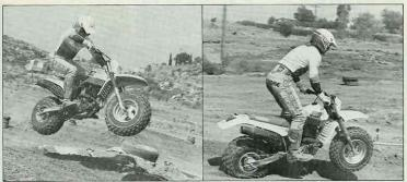
Flight time is fairly neutral as long as the takeoff ramp is straight. Thanks to an improved suspension system, landings are better absorbed on the 350 than the 200. Check out the ripples in the rear tire.
