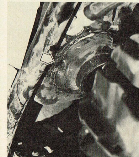
By pushing lightly with your finger you can leave a dent in the rubber air boot that will leave an opening into the air box.
