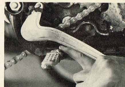
Rear brake pedal provides no height adjustment and is only a finger away from the frame tubes when engaged before you start to ride.
