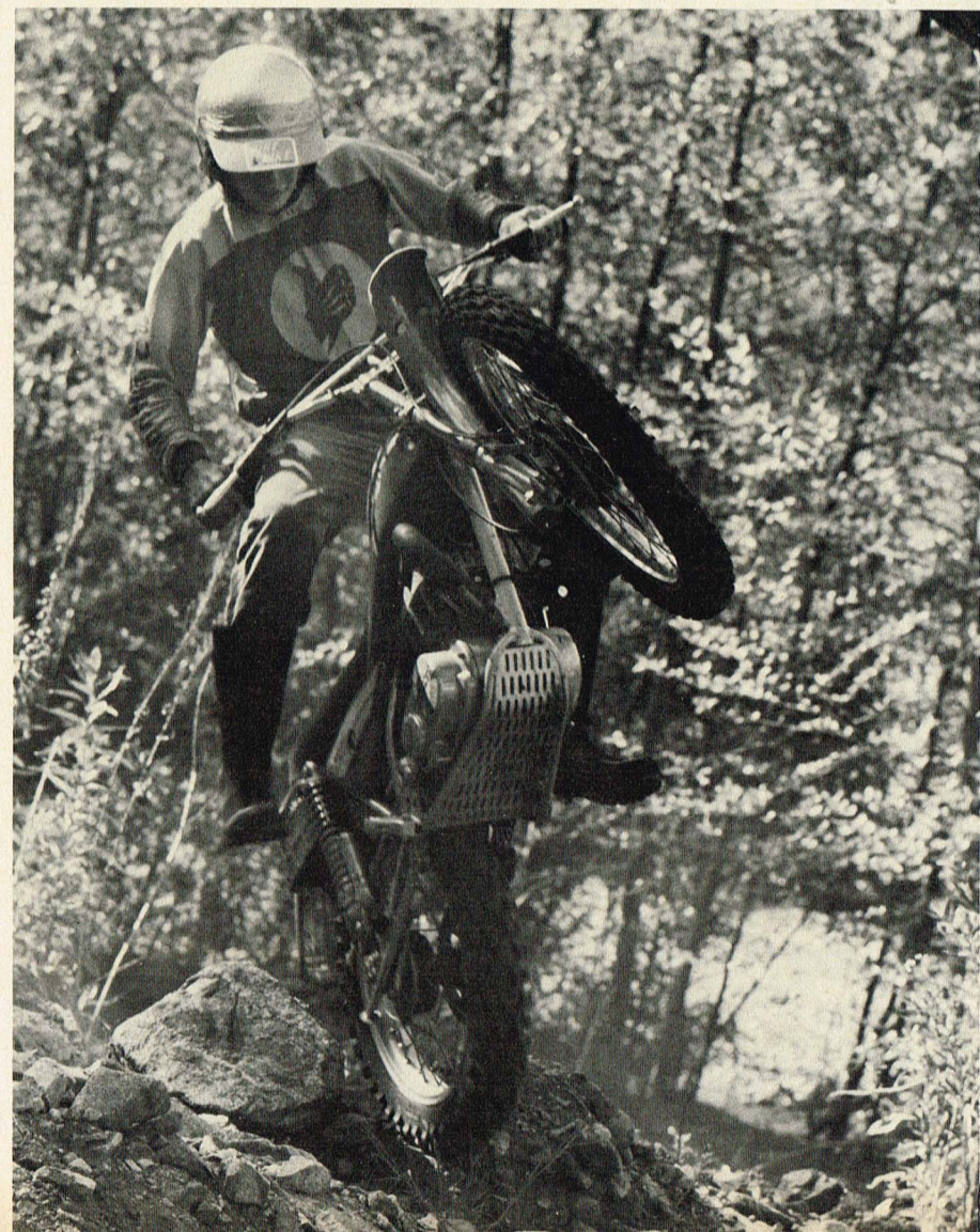
Light hubs, with chrome brake liner. Notice similarity to '75 Pursang. Buddy pegs added for Alpina. Betor shocks have heavier springs than Sherpa (about 55-75 progressive to the T's 55-pounders), adjustable air reservoir. Same spark arrestor as T, still not stamped USFS-approved, although there are numbers on them. It's a very quiet bike.
