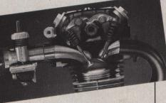
Kerker Stage III system featuring the Kerker flow perfected head. A 24% flow increase across both valves is achieved with this setting.
