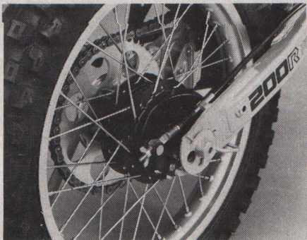
A quick-release brake cable and an axle puller welded onto the axle speed repairs.
