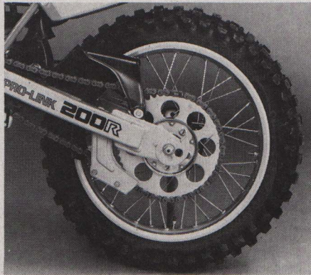
A sturdy chain guide, chain guard and slider keep the XR sailing smoothly.
