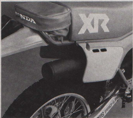
An effective spark arrester/silencer combo keeps the noise down to 98 dbA.
