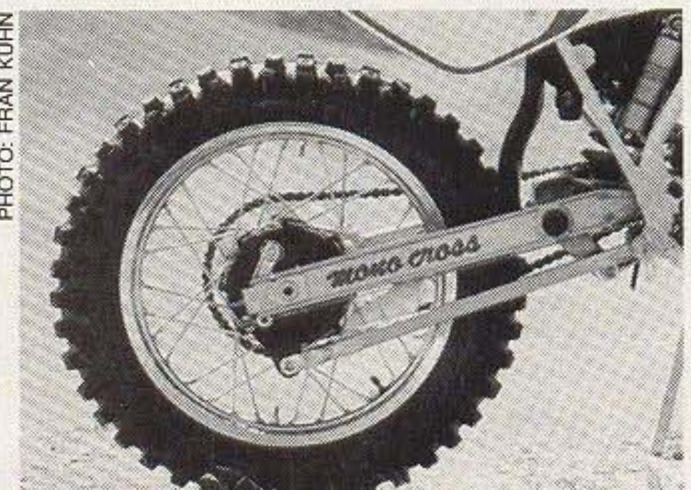
The new bleed-style shock is more compliant on the smaller bumps, even with a nearly flat leverage curve.
