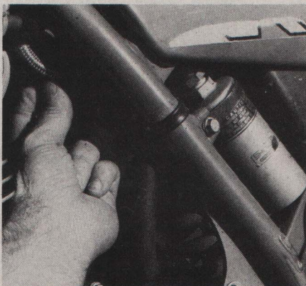
The White Bros. braided stainless steel hose and rubber bump stop are added: Only a class A rider needs the stiffer XR250R spring.
