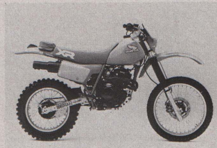
The popular XR500R and XR350R models received updates such as handlebar brush guards and a change in the material used in the chain guide. The 500's (left) fork was modified for smoother action, while the 350 (right) got a front disc brake this year. Forks on both bikes (41mm for the 350, 43mm for the 500) deliver 11 inches of travel. Pro-Link suspension, with adjustable rebound and compression damping, delivers 10.6 inches of rear wheel travel on the 350 and 11 inches on the 500. Dry weights are 247 pounds for the 350 and 267 pounds for the 500.
