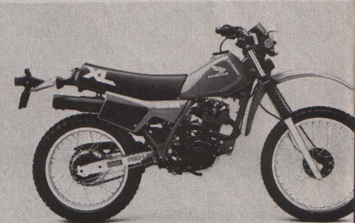
Honda also introduced a pair of new dual-purpose bikes. The XL250R (above) puts the promising new 249cc RFVC motor into a dual-purpose chassis with 8.7 inches of front wheel travel and 7.5 inches at the rear. The XL350R (above right) is the street-legal version of last year's hit single, the XR350R. The XL350R claims 8.7 inches of front wheel travel through a 39mm fork and 8.1 inches at the rear wheel through Pro-Link suspension with adjustable rebound damping. The 350 also gets a disc brake up front.
