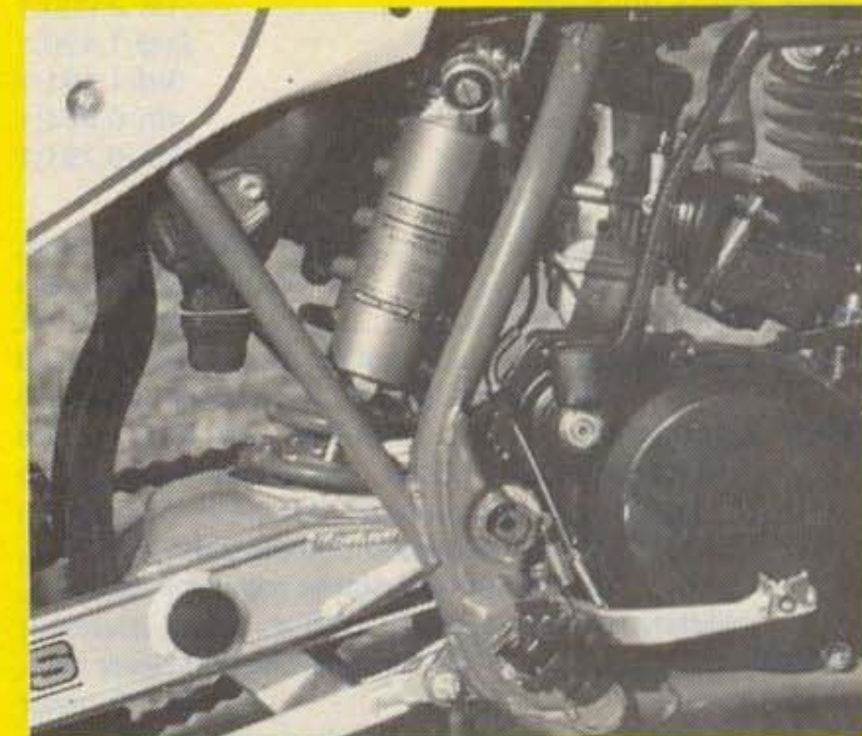
The new Monocross linkage works well enough to provide the best suspension in the Open class... stock!
