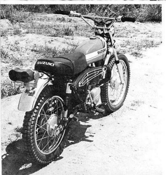
The Sierra is very slender and the exhaust system is tucked well in and covered by a chrome guard to protect the rider's leg.
