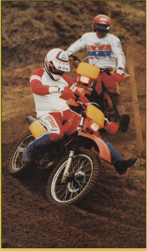
Plastic work on both bikes is red, with hand guards this year's bonus. However, the 250 comes with a smaller fuel tank. With a nine litre capacity, it is three litres down on the 350. Other similarities include the nifty quick change rear wheel system, sidepanels which hide the oil foam air filter - which are different - and the engine decompression levers.
