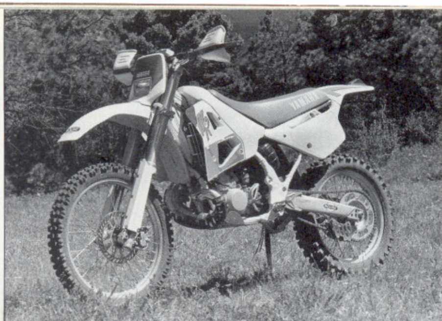
With a little work, the WR200 headlight and front fender will go onto the 250, giving it a very different overall personality.
