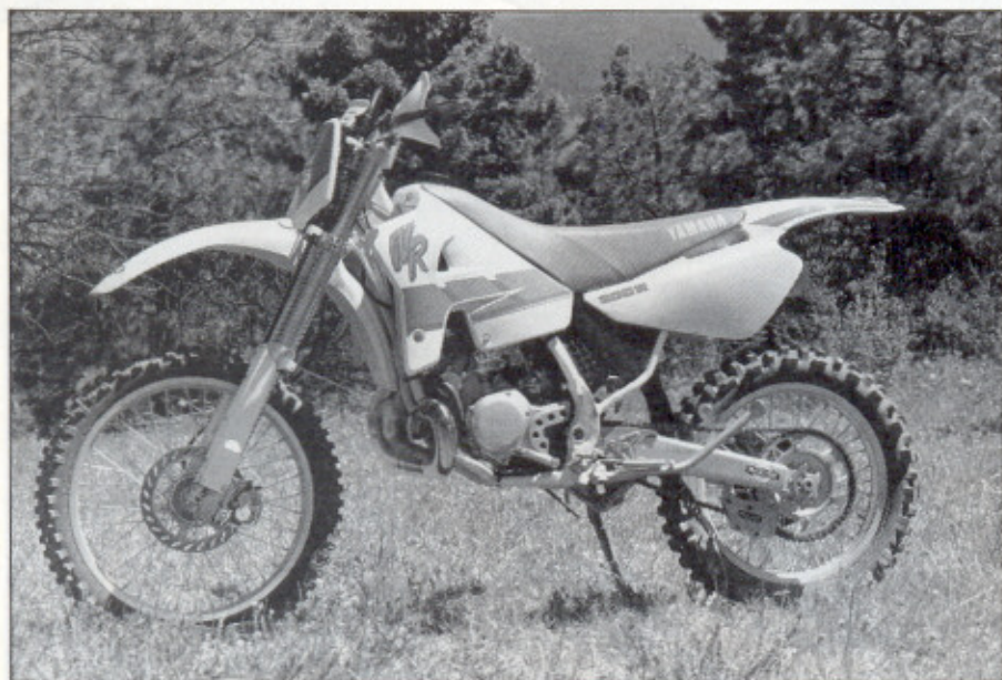
The FMF pipe and Answer silencer provided a lot of the horsepower gain for the 200. The rest was through hard work and grinding.
