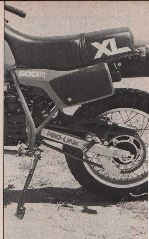
The XL's Pro-Link system features adjustable damping and pre-load. Cleverly designed helmet lock also locks the tool kit. Rad!
