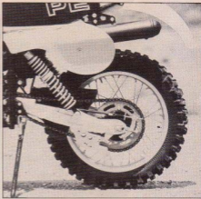
The entire rear end is new, with a true quick-change wheel, an extruded aluminum swingarm, and over 9 1/2 inches of wheel travel.
