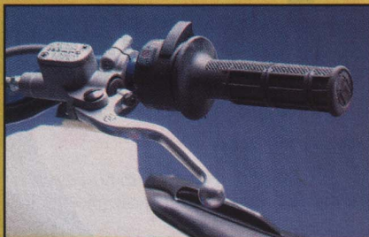
TM was using hydraulic clutches before KTM, Billetanium or any of the others.
