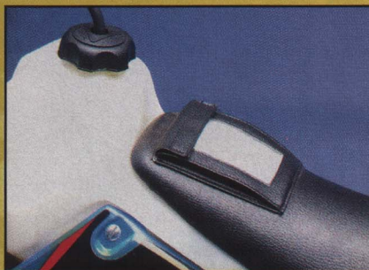
Need a place to keep your change? European enduros have time clocks; hence the easy-access card pocket.
