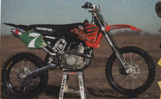
Thumper's 94mm piston brings displacement to a 2003-legal 447cc, while the 95mm piston kit yields 453cc. The TR cam adds boost across the board, too.
