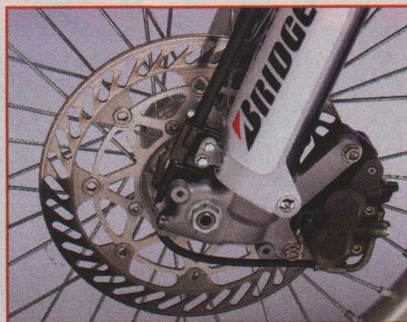
Bubba's magnesium brakes aren't much more powerful than stock, but they are considerably lighter.
