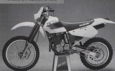
With RM-grade brakes, swingarm linkage and fork, the DRZ250 has a lot of ground control. Like with past RMs, only the left subframe is removeable. The other offerings come with handguards, but not the DRZ.
