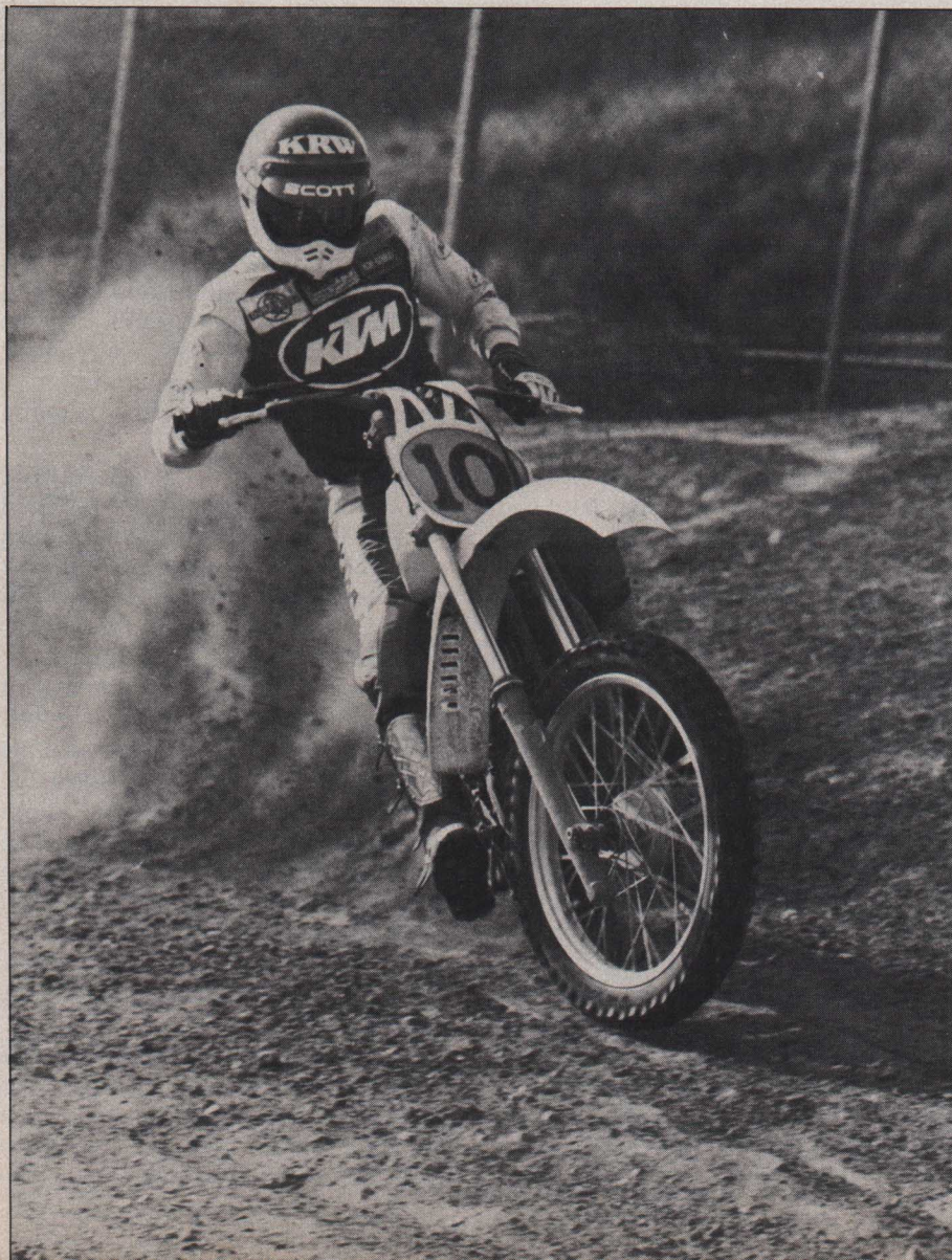
Super Ohlins shocks came standard on the 495. Spring rates were spot on for the average 150-pound rider.
