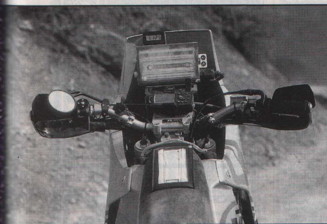
The Dakar 660 has almost as many things to look at and play with as a private airplane. Competitors live by the route chart (complete with handlebar-mounted advance/reverse switches). The GPS has a remote control also.
