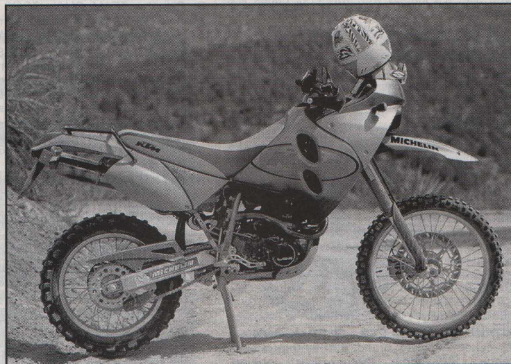
It's not a naval vessel, it's an Adventure R. The A-R carries 7.4 gallons of fuel and has a 48mm fork off of the Dakar 660.
