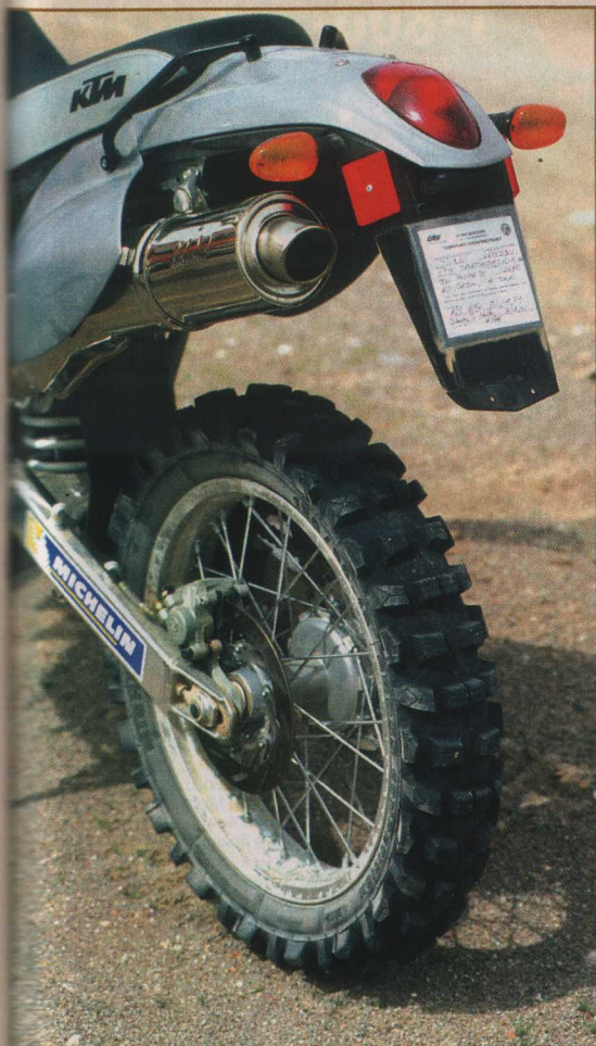
The stainless muffer has a pre-chamber and the spark-arresters are enclosed midway in the cannister. This makes the back portion a resonator chamber, ala AMA dirttrackers. They may see you, but they'll never hear you!
