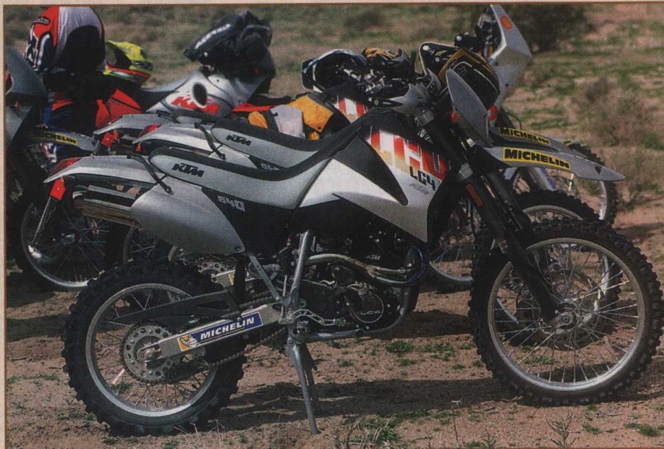
The stainless muffer has a pre-chamber and the spark-arresters are enclosed midway in the cannister. This makes the back portion a resonator chamber, ala AMA dirttrackers. They may see you, but they'll never hear you!
