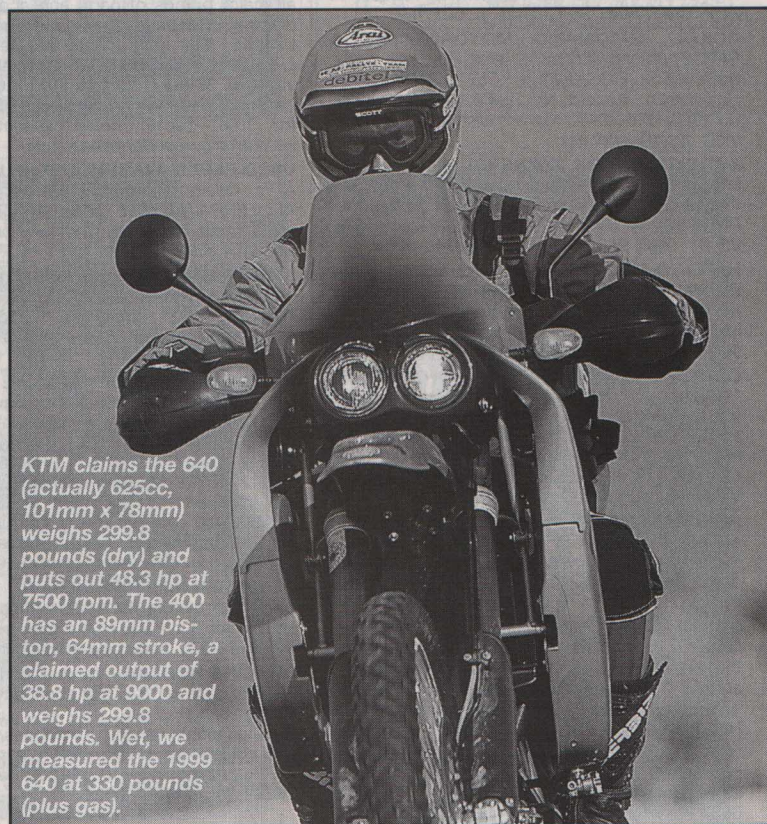
It's not a naval vessel, it's an Adventure R. The A-R carries 7.4 gallons of fuel and has a 48mm fork off of the Dakar 660.
