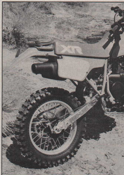
An aluminum swingarm replaces the steel unit of years past. A revised shock has easier-to-reach rebound adjuster and grease fittings on the linkage. The powerplant shows no external changes. But inside you'll find a bigger hole, more torque and a changed oiling system.
