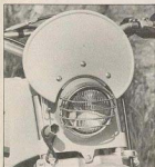
Tidy front end has a lot of neat, small features: rock guard over headlight, raised number plate and multi-purpose, quick-disconnect tool.
