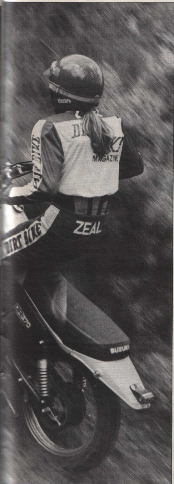
The short, metal rear fender and the seat which widens at the rear to accommodate it are examples of the DR's styling getting the upper hand on function.
