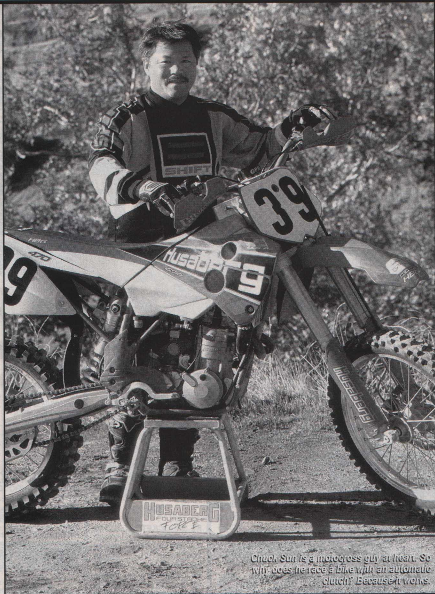
A Husaberg FC470 is odd enough in stock trim, with a cylinder casted into the engine cases.
