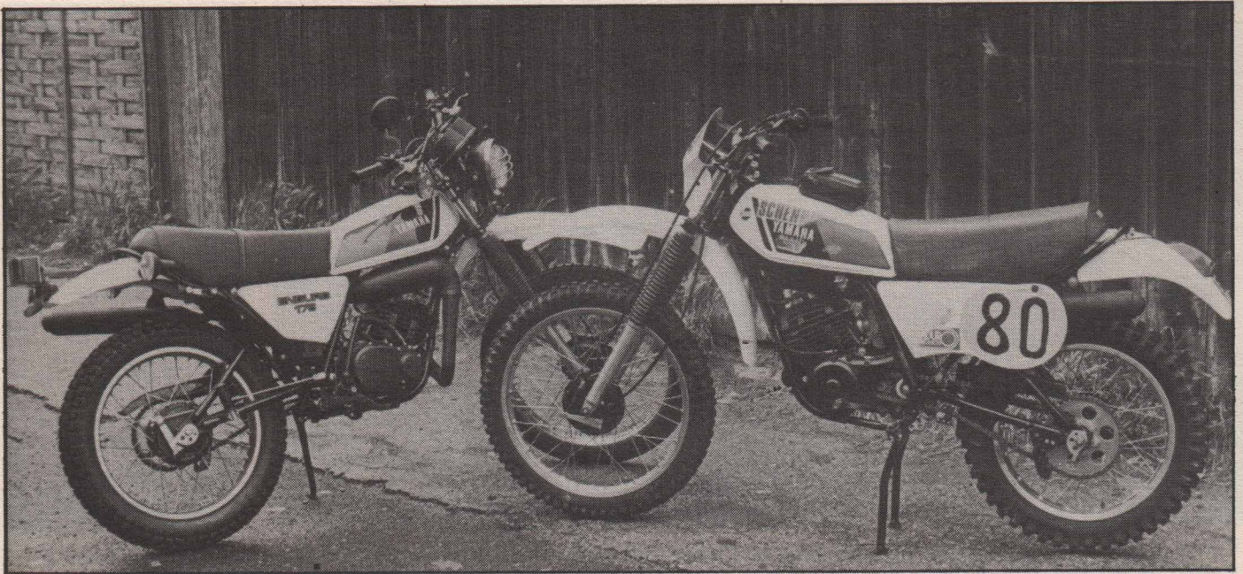
The two bikes may look pretty similar, on first inspection, but Rayner's modified machine on the right is considerably lighter, and quicker! Note, too, his choice of a centre-stand — much easier for rear wheel removal out in the trails.
