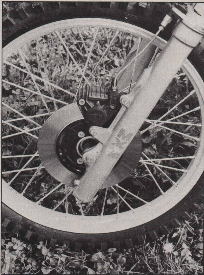
Powerful Brembo disc brake really hauled the 495 down from speed. It was unaffected by water or mud. New 42mm Marzocchi forks are primo.
