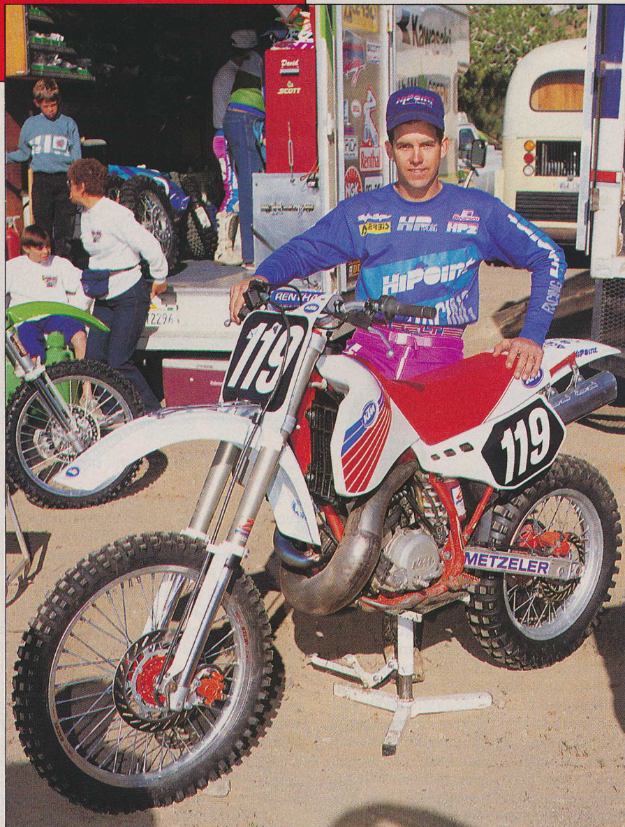
The 1990 KTM 250 requires 92 octane or better, so unleaded premium or regular fuel with an octane booster is needed for good engine life. Dan Smith and other top KTM off-road pilots use racing fuel for a winning edge.
