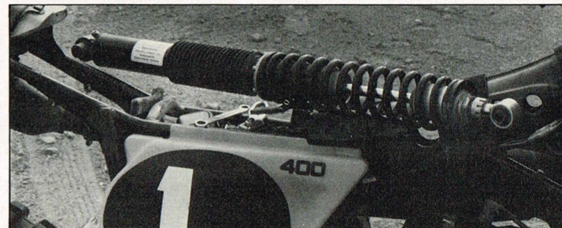
Bare naked. Collar on right near shock eye rotates to adjust dampening force. The nut to its left can be cranked up or down to change preload settings.
