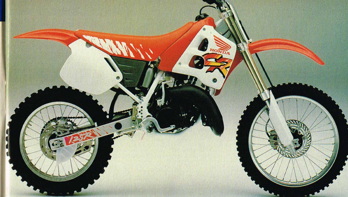
◀ New linkage ratios and damping curves, graphics and 250-styled gas tank, seat, side panels, rear fender, airbox and subframe highlight the 1991 CR125. Honda's press release says the "striking new graphics emphasize the aggressive performance of the hot new CRs."
