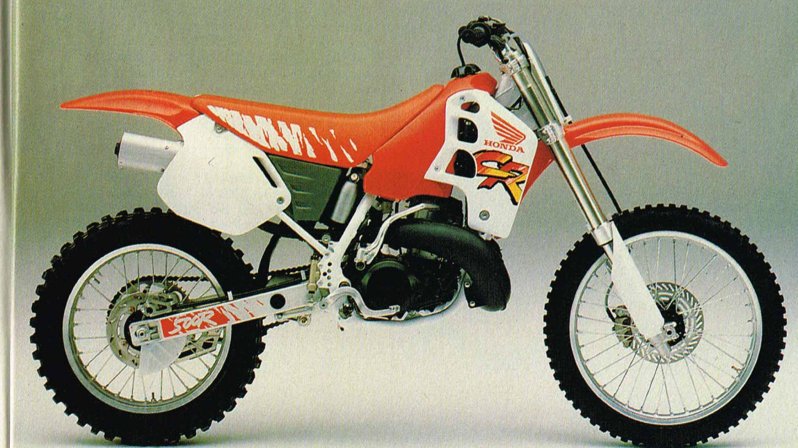
◀ Like the 125 and 250, the CR500 gets a new KYB shock with a newly developed swivel bearing. The 500 also gets 250-styled subframe, airbox and plastic. Numerous refinements grace all three red rockets.
