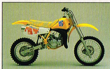
The best 80 of '90 gets better for '91. Its modifications are intended to make it more fun and easier to ride and less a pain for dad to maintain. Additional gusseting behind the steering head increases rigidity.
