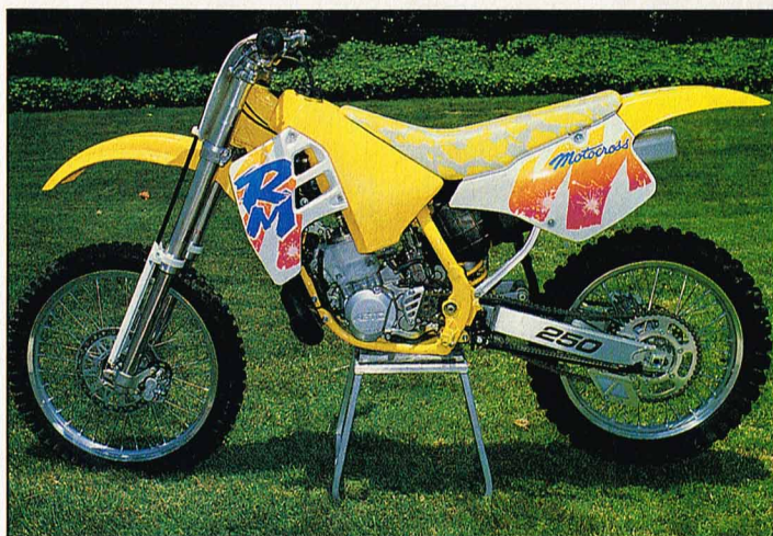
More frame rigidity, quicker turning, completely new Showa suspension, more powerful brakes and across-the-board power increases were the goals for the 1991 RM250. We hope it's as fast as it is ugly!
