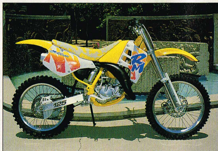
For the last two years, the RM125 has been a slug on top-end. Suzuki set out to change that with a less-restrictive silencer, exhaust boost ports, new exhaust valve guides and new piston.
