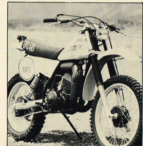
The RS features a PE250 motor—six-speed tranny and plenty of torque.
