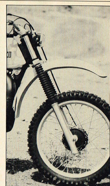
Front forks are also '79 PE style, with 9.1 inches of travel and no air caps. Action was a little on the soft side, but very good over the bumps.
