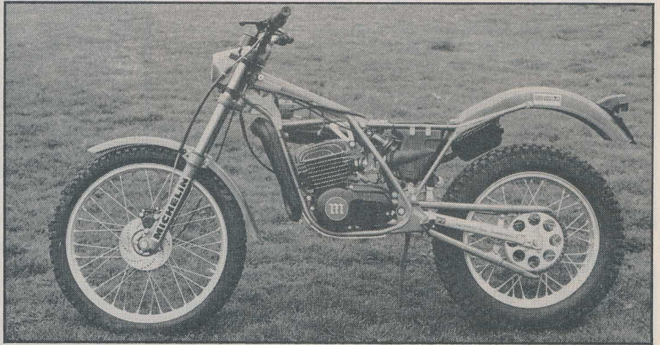
Redesigned frame has completely detachable rear subframe for good suspension access. Top and bottom chain guards are used for extra protection. Montesa's first disc front brake is effective.
