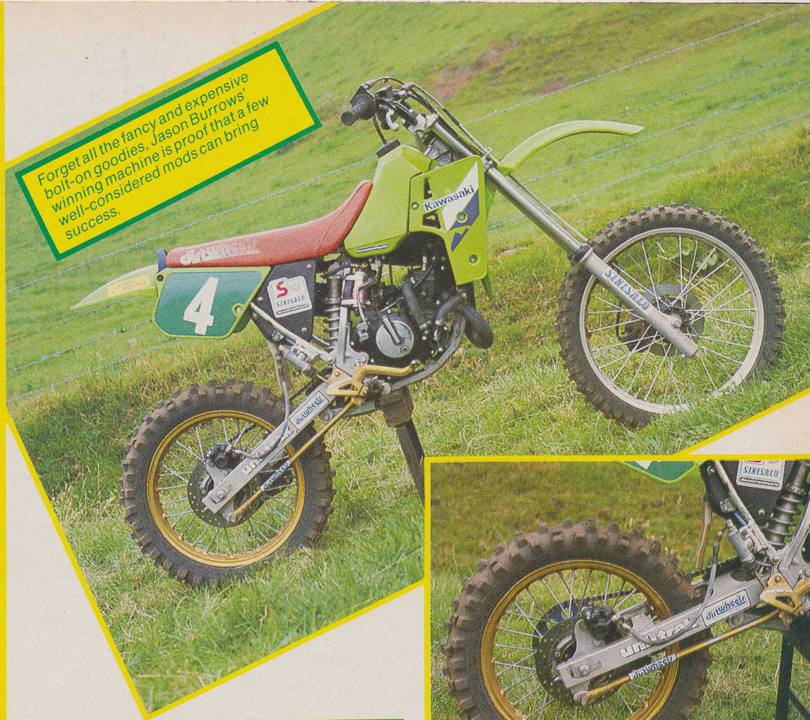
The ultra trick rear disc brake. It's Dirt Wheels' own conversion.
