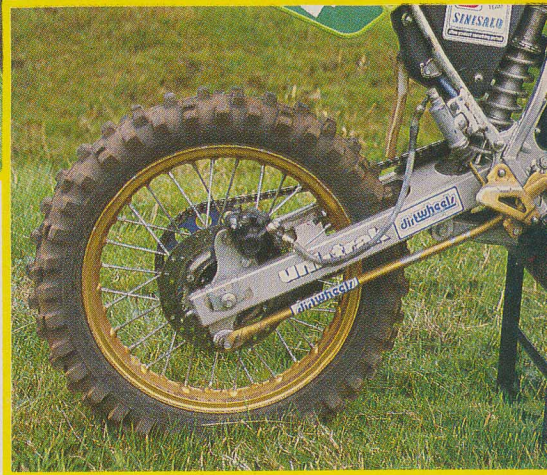
The ultra trick rear disc brake. It's Dirt Wheels' own conversion.
